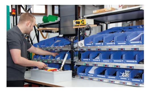
When it comes to manual mounting in industry, it is important to work precisely, quickly and accurately to ensure the quality and safety of the end product and to ensure that deadlines are met. A pick-to-light system from KBS can provide efficient support in this regard to ensure competitiveness.
